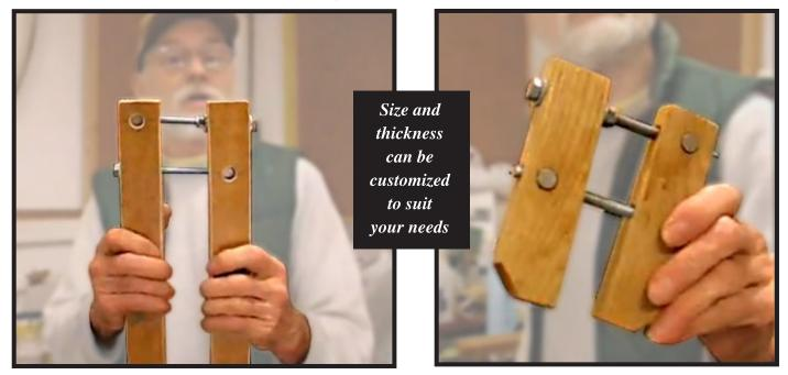
**Description** These are inexpensive, simple clamps for situations where you need to attach gunwales and outwales, or for hard to reach places. Jaws can be hardwood, softwood or plywood depending on use. To operate, roll the bolts in your fingers to open/close the jaws together. It depends how you hold the clamps (which side is up), as to which way the jaws move when you roll the bolts. A description is included in Red Barn Boats YouTube videos:
